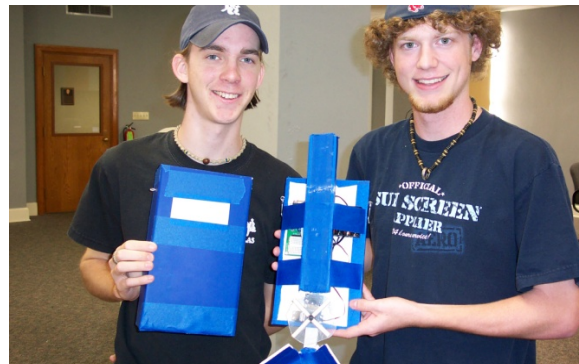
poker chip sorter - uses color sensor
