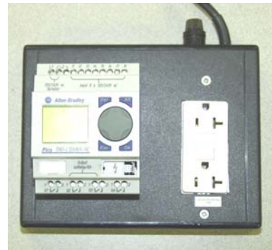
Figure 2: Mounted PLC Unit.
