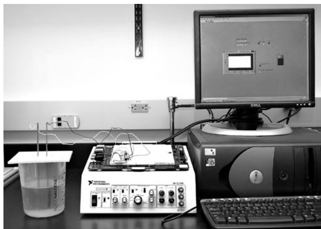
Figure 5. Capacitive liquid level meter instrumentation system. Parallel copper plates immersed in oil are connected to a 555LM oscillating circuit on a NI-ELVIS station. A PC running LabVIEW is used to acquire the oscillator frequencies, analyze the signal, and display the relative liquid level on the front panel.
