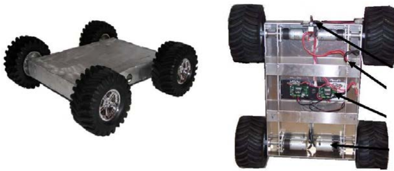
Figure 2. Top and Bottom Views of the Robot Base.
