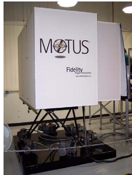
Figure 8. The WVU 6 – DOF Flight Flight Simulator Cabin.
