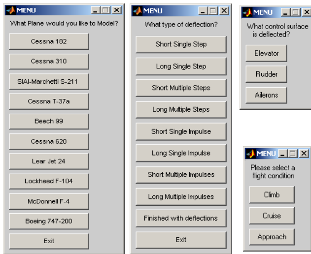
Figure 2. Matlab Interface for Handling Qualities Evaluation Using Transfer Functions.
