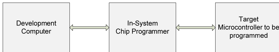
Figure 2 – Overall Block Diagram of an In-System Programmer Setup.
