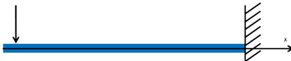
Figure 1. Cantilever beam under concentrated load.
