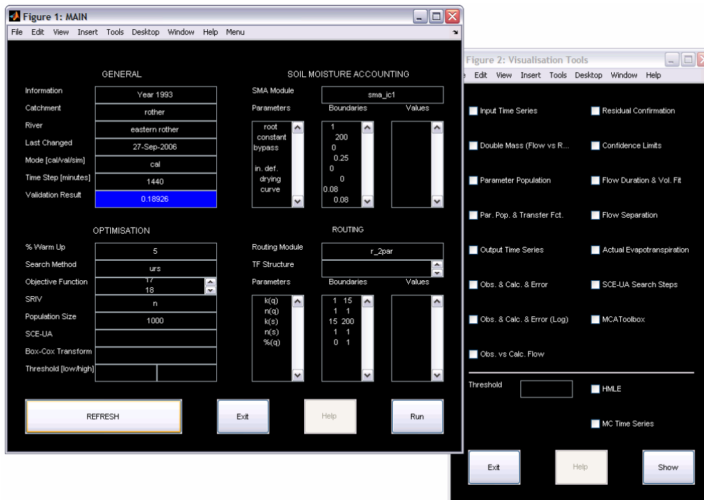
Figure 3. GUI of the Rainfall-Runoff Modeling Toolbox (RRMT) consisting of two parts, the main GUI and a visualization GUI.
