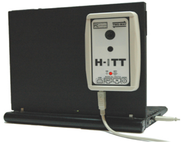
Figure 2: Base Unit attached to Notebook Computer via USB[2].
