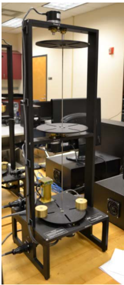
Figure 3. ECP experimental modules (a) Rectilinear System, (b) Magnetic levitation, (c) Torsional system, (d) response of the torsional system bump test for the system identification experiment.
