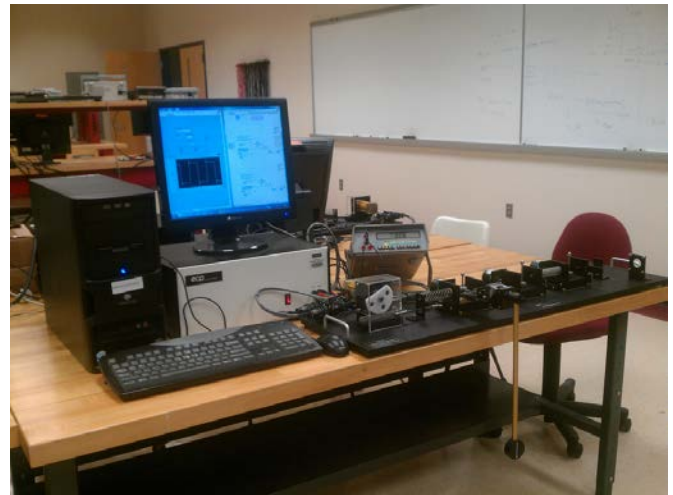
Figure 5. Experimental setup for position control of a cart-pole system.
