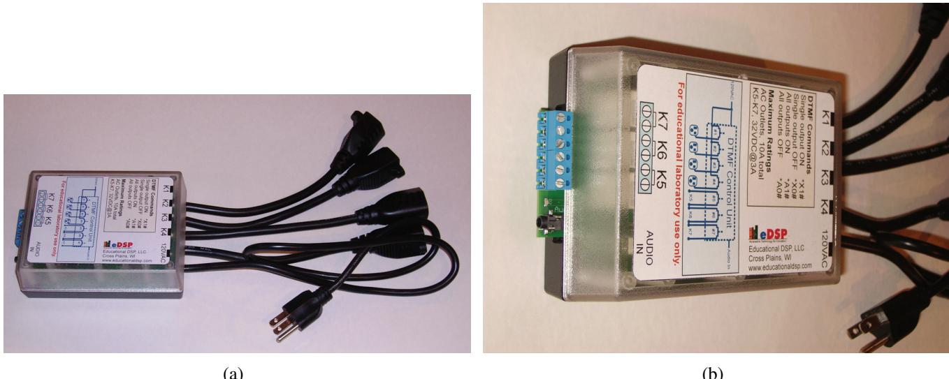
Figure 5: The new DTMF decoder and power switch box that allows various appliances to be controlled via DSP. (a) The AC power line for supply to the unit and the four AC connectors for controlling external appliances are shown. (b) The three low-voltage relay connections and the audio signal (DTMF) input connector socket can be seen.
