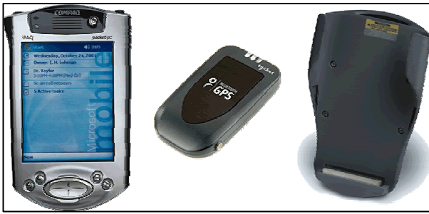
Figure 1: iPAQ H3970 (Left), Socket Bluetooth GPS Receiver (Center), and Symbol SPS3000 Barcode Scanner Sled ( Right).
