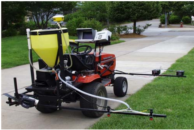
Figure 2. Weed detection system with variable rate applicator.
