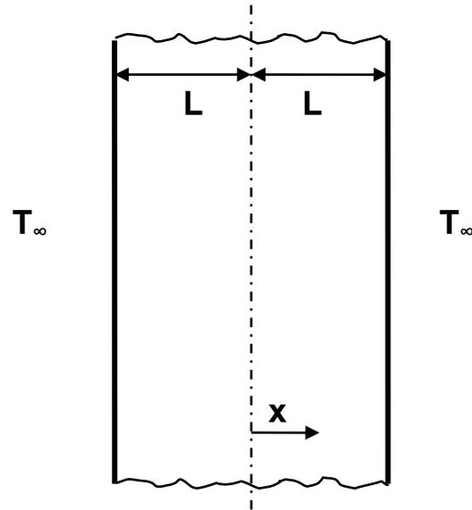
$$\theta^* = \frac{T(x, t) - T_\infty}{T_i - T_\infty} \quad x^* = \frac{x}{L} \quad t^* = Fo = \frac{\alpha t}{L^2}$$
